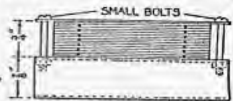
Fig. 19.—Method of Clamping Transformer Together
