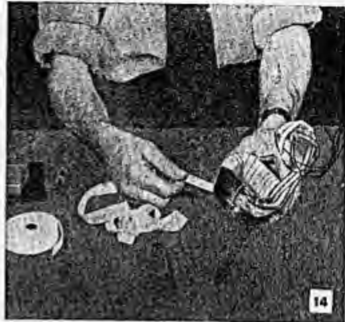
Completed coils are taped together with white cotton tape. Remove the tie strings as tape approaches them
