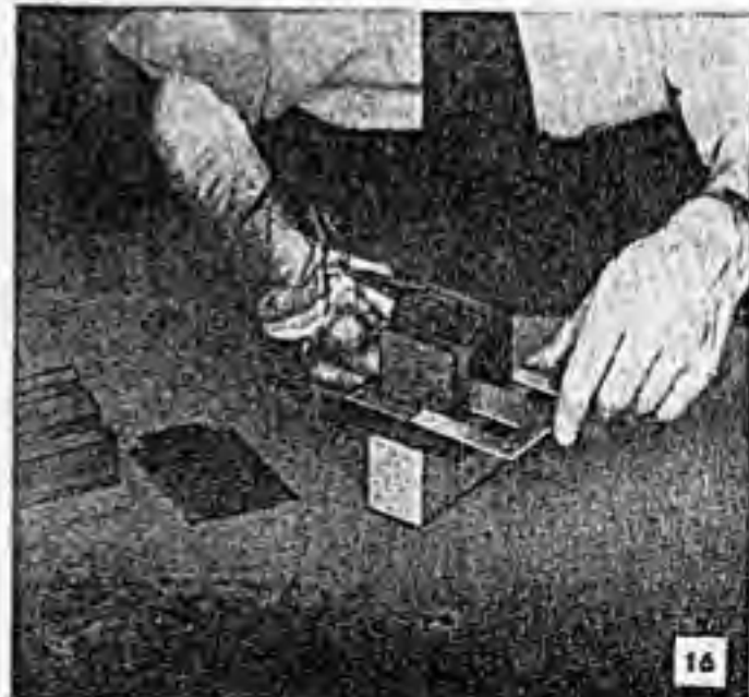
In assembling core and coil, alternate positions of the straight and E-shaped laminations from side to side
