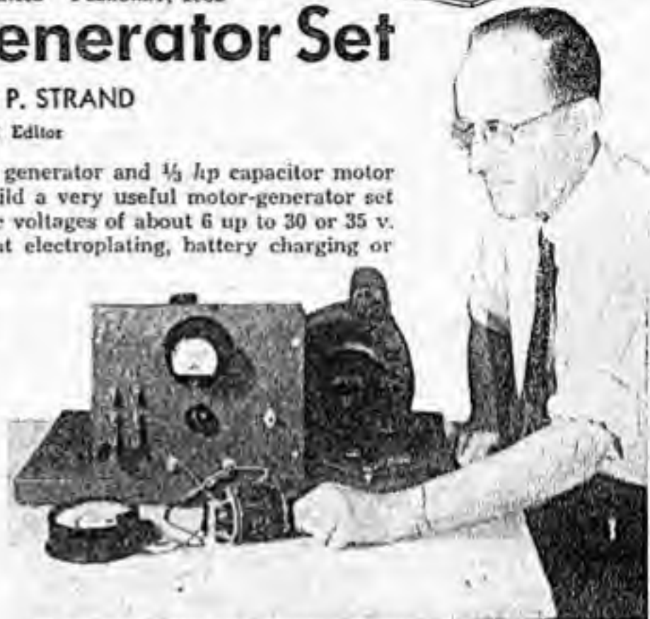
The motor-generator set delivering 28 volts dc to a surplus dynamotor, from which 220 volts dc can be obtained.
